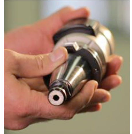
Example of a toolholder with a coolant hole
